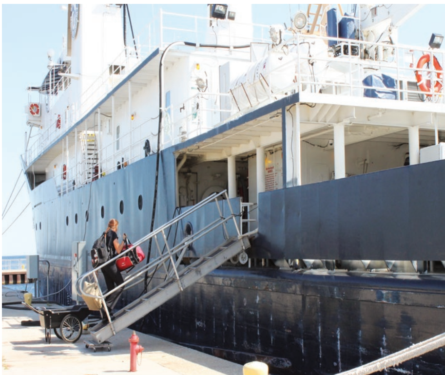
Engineering cadet Tess Lepley reports aboard the 224-foot former U.S. Navy submarine surveillance ship Persistent , which is now T/S State of Michigan . The vessel was built in 1986 and designed to tow highly sensitive sonar arrays for tracking Soviet submarines.
