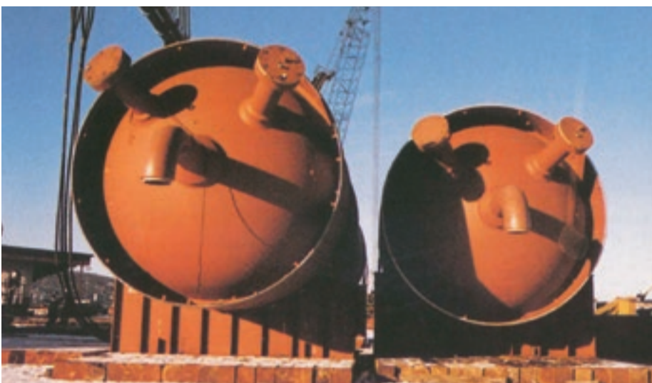
Two massive oil refinery reactors, weighing 750 tons each, await transport at the Clure Public Marine Terminal in 1987. They were part of the Great Lakes’ heaviest lift project at the time.
