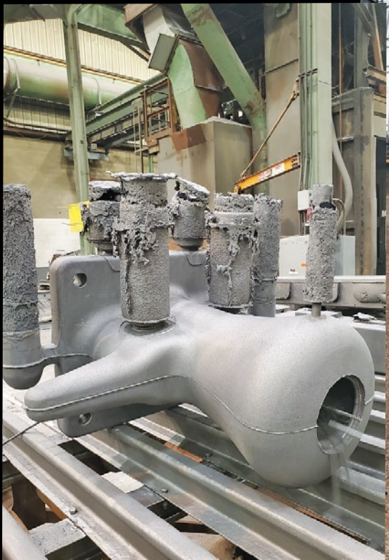
Once the metal has cooled, which can take up to 72 hours, the bollard is put on a conveyor belt for the shot blast process. This removes any debris or stray bits of metal, creating a sleek finish.
