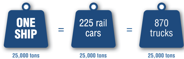
A maximum Seaway-size laker can carry 25,000 metric tons per voyage, the equivalent of 225 rail cars or 870 semi-trailer trucks.
