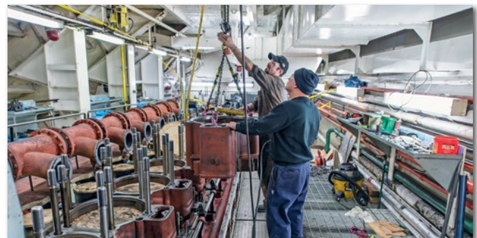
On the Edwin H. Gott , Michael Kolenda (foreground), Great Lakes Fleet engineer, and Aurel Carina, MaK service engineer, remove heads from the starboard main engine as it undergoes a complete overhaul, part of routine winter maintenance.
