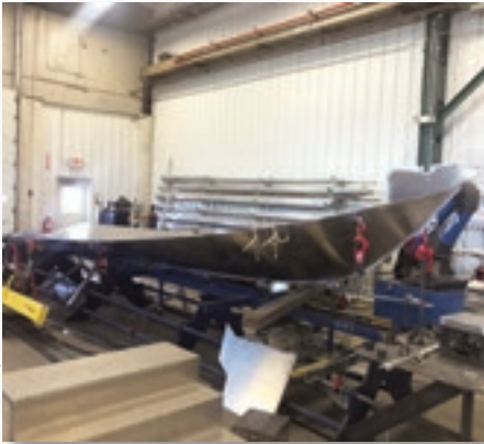
The bottom hull shell is fit to the keel.
