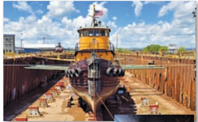
Two Heritage Marine tugs in dry dock at Fraser Shipyards for inspection and repairs.
