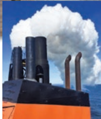
Interlake's signature white clean steam plume will be visible from the stack of the Paul R. Tregurtha once her scrubbers are installed this winter. [Inset courtesy Interlake Steamship Co.]
