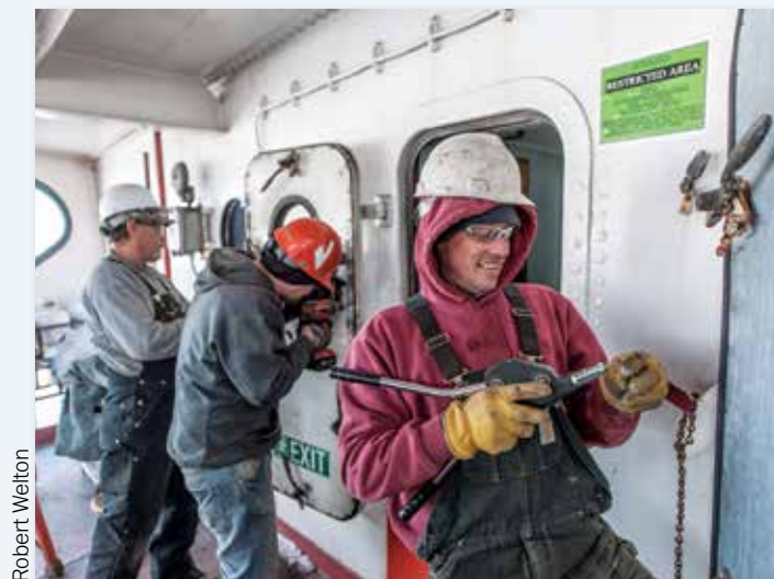
A winter work crew hired through Key Lakes Port Services works on re-fitting gaskets on all water-tight doors and portholes aboard the Phillip R. Clarke . The trio tackling that task during layup at the end of last season included (from left) Mark Beals, Travis Avey and Rob Seagal.
