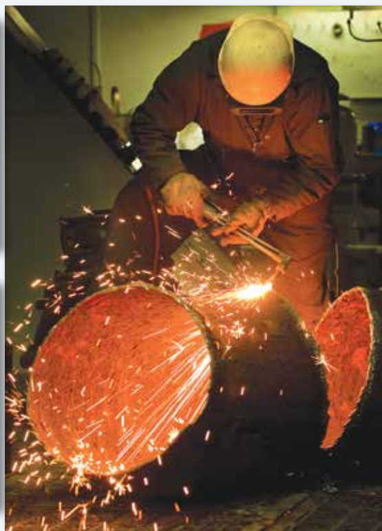
A pipefitter cuts an old ballast pipe section being replaced in a freighter.
