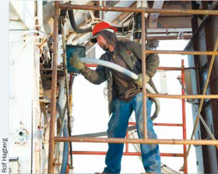
Jason Glaus replaces one of the boom motor feeders from the controller and resistor grid on the John G. Munson .
