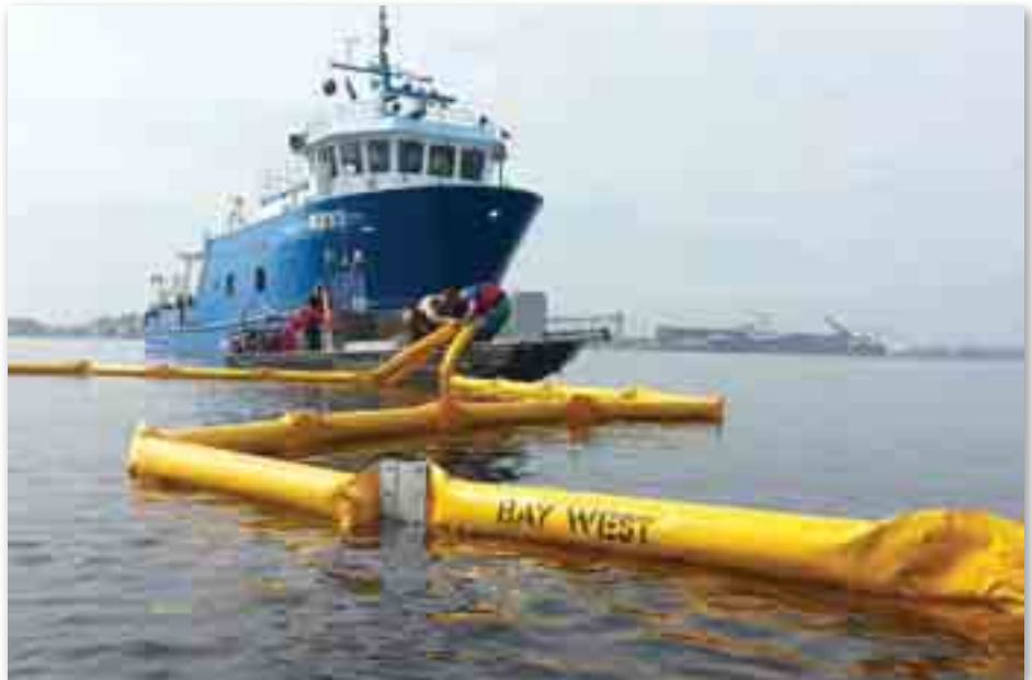
Pollution-containment equipment is placed around the Kiyi during a Coast Guard training exercise.
